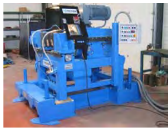
Beveling Bench BB 3" – 16" 88,9 mm – 406,0 mm 12" – 24" 323,9 mm – 610,0 mm
